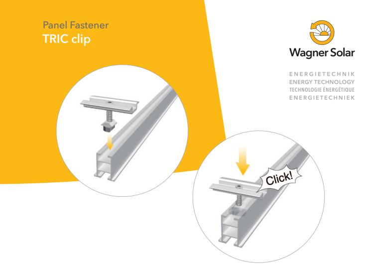
The TRIC about the Clip - for fast and safe panel installation. A flick of the hand, and the TRIC clip panel fastener automatically snaps into the right position, confirmed by an acoustic signal. Fits with all TRIC on-roof and free standing systems.
