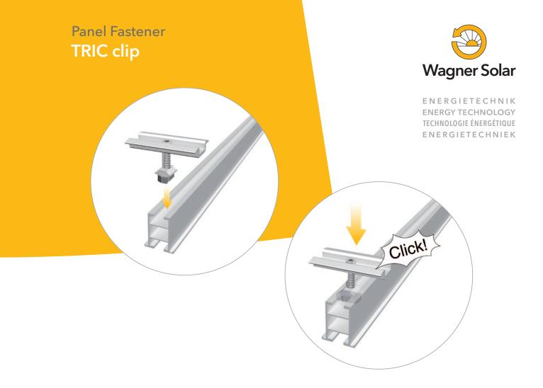
The TRIC about the Clip - for fast and safe panel installation. A flick of the hand, and the TRIC clip panel fastener automatically snaps into the right position, confirmed by an acoustic signal. Fits with all TRIC on-roof and free standing systems.
